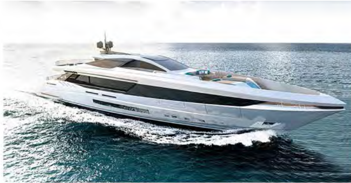
The GranSport 45 is set to include three MTU 16V M96L engines, two of which connect to a fixed-pitch propeller shaft, and a third of which connects to a Rolls Royce waterjet. The propulsion system will allow the superyacht to reach a maximum speed of 26 knots and a cruise speed of 11 knots. Furthermore, all three engines comply with IMO Tier II and EPA Tier III emissions regulations.
