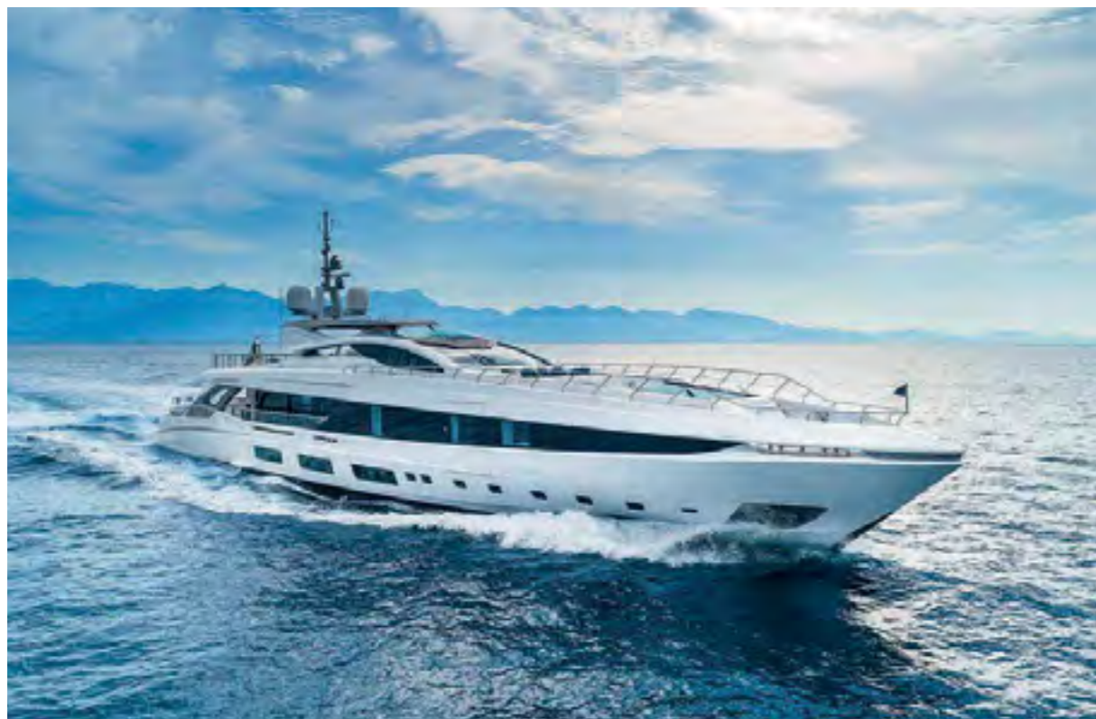
A surface-piercing hull by PLANA coupled with 10,400hp from four MTUs gives this 54m a top speed of 30 knots. Cruising at 14 knots, she crossed the Atlantic in six days – the first Mangusta ever to do so
