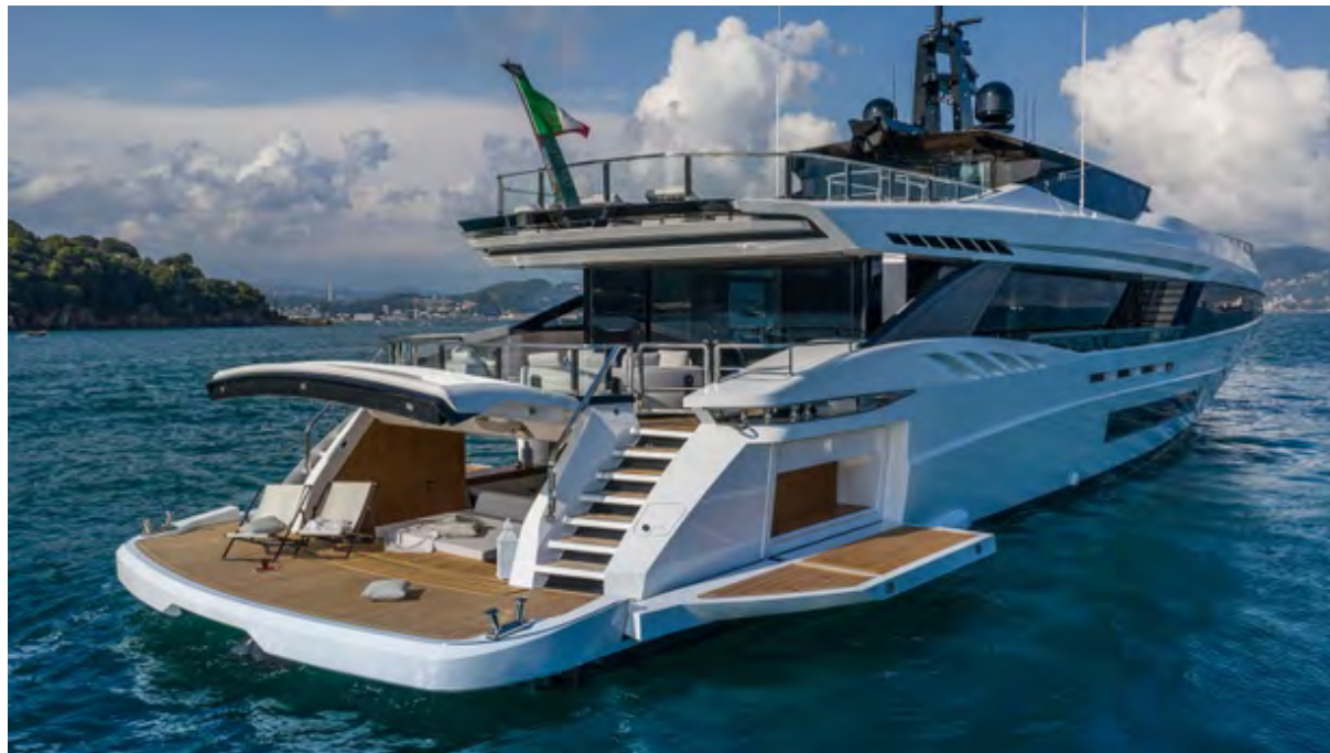
The beach area consists of three interconnected platforms: two terraces rotate from the side connecting with the central platform and creating 75 square metres of useable area in direct contact with the sea
