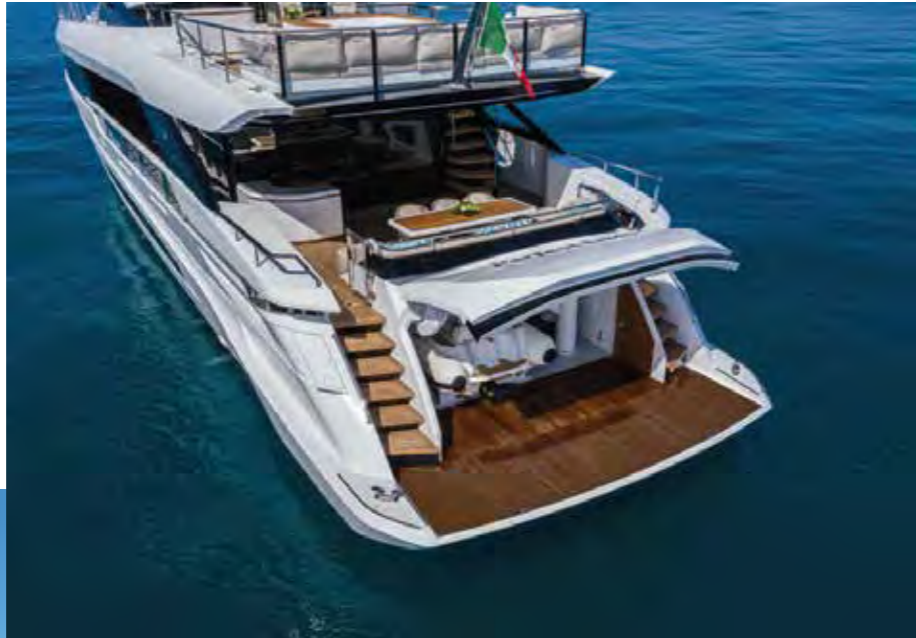
Right: twin staircases frame a garage that can hold a tender of up to 5.4m in length – or whatever toys the owner chooses
