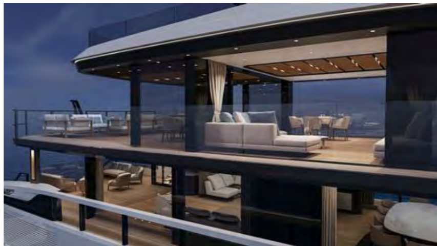
Highlighted features include minimised bulwarks, glass handrails and ceiling-high sliding glass doors
