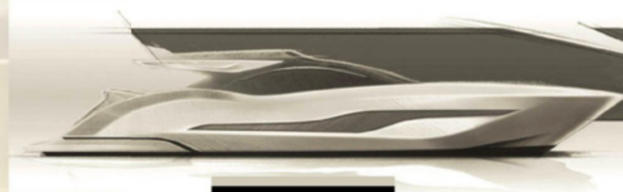
Instead of portholes on the lower deck, the 104 REV features a continuous expanse of dark glass that emphasises the hull's curves
